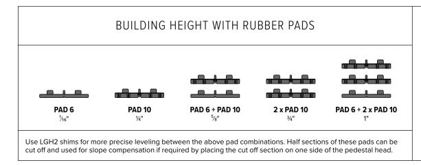
ETE-PAD 6 and ETE-PAD 10 components are stacked to build paver support up to the height where PR1, the lowest adjustable height pedestal ( $1 \frac{3}{16}$ "-  $2 \frac{1}{2}$ "), can be used. LGH2 shims are used to make minor height adjustments as needed.
