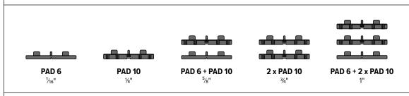
Use LGH2 shims for more precise leveling between the above pad combinations. Half sections of these pads can be cut off and used for slope compensation if required by placing the cut off section on one side of the pedestal head.
