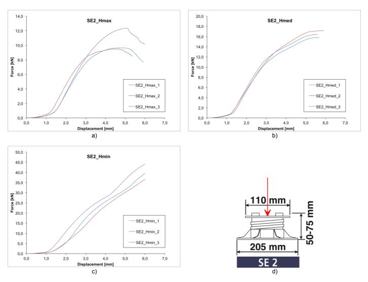
Figure 1 Diagram force versus displacement of testing machine's crossbar for Hmax (a), Hmed (b), Hmin (c) and typical "Eterno SE2" specimen (d).
