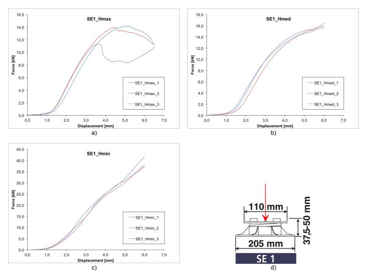
Figure 1 Diagram force versus displacement of testing machine's crossbar for Hmax (a), Hmed (b), Hmin (c) and typical "Eterno SE1" specimen (d).
